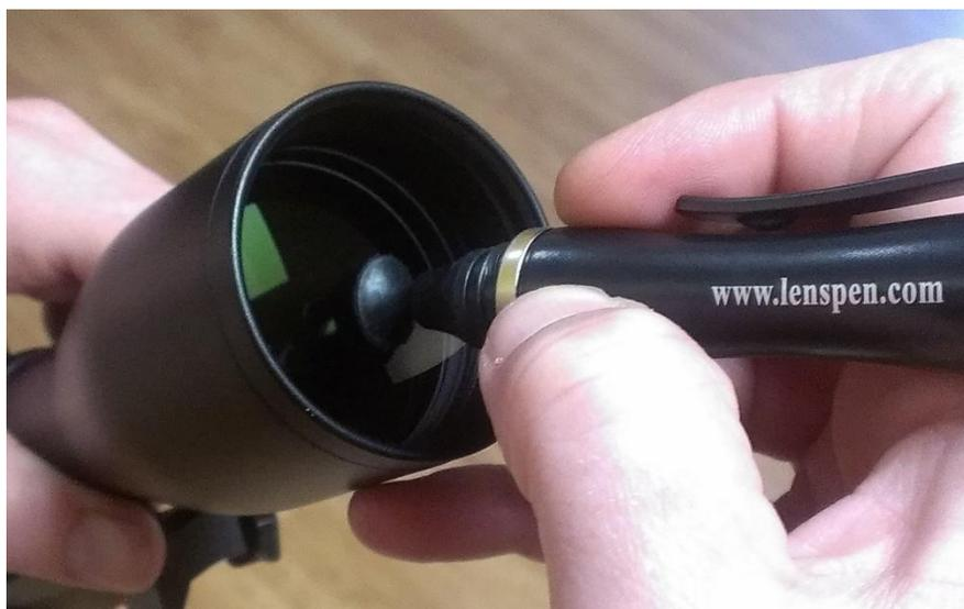
**Fig 4 Carbon compound impregnated cups remove any last streaks and oil.**
