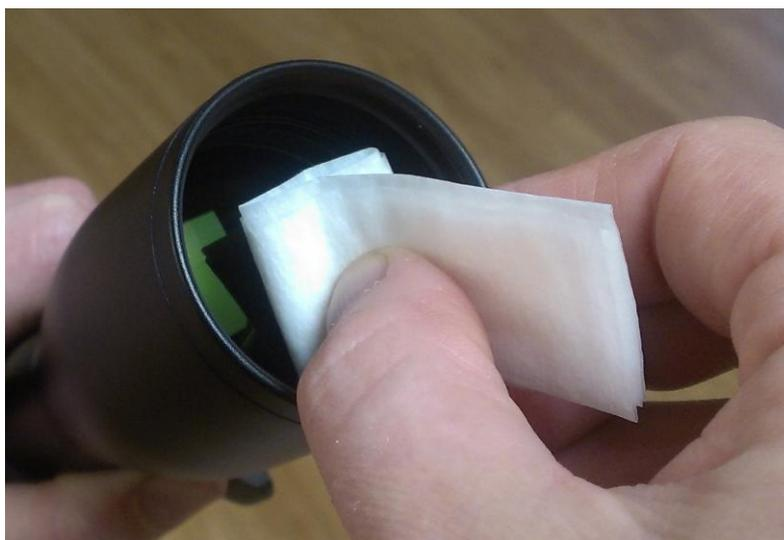
**Fig 3 Proper application of disposable lens cleaning tissue.**
